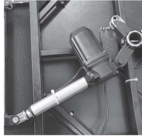
Incorrect position of the rotation motor
