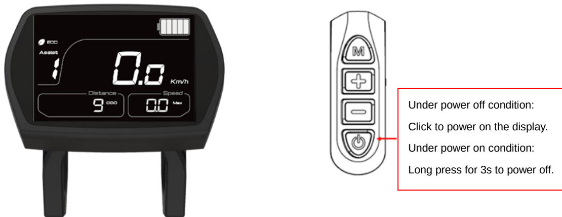
Figure8-1 Power on/off operation
