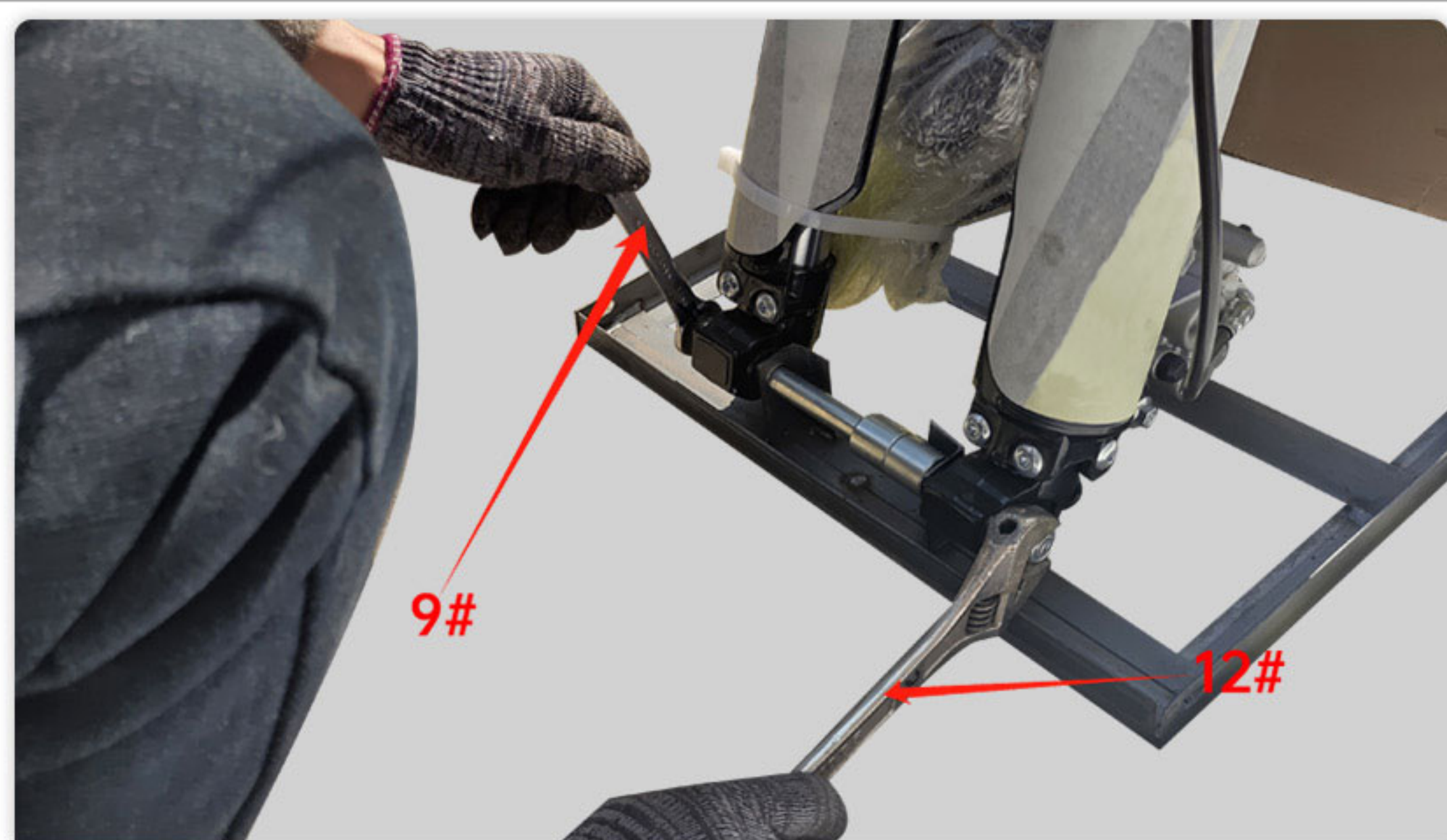
8. Using 5# 12# tool disassemble the front axle and put the front axle and spacer to next using
