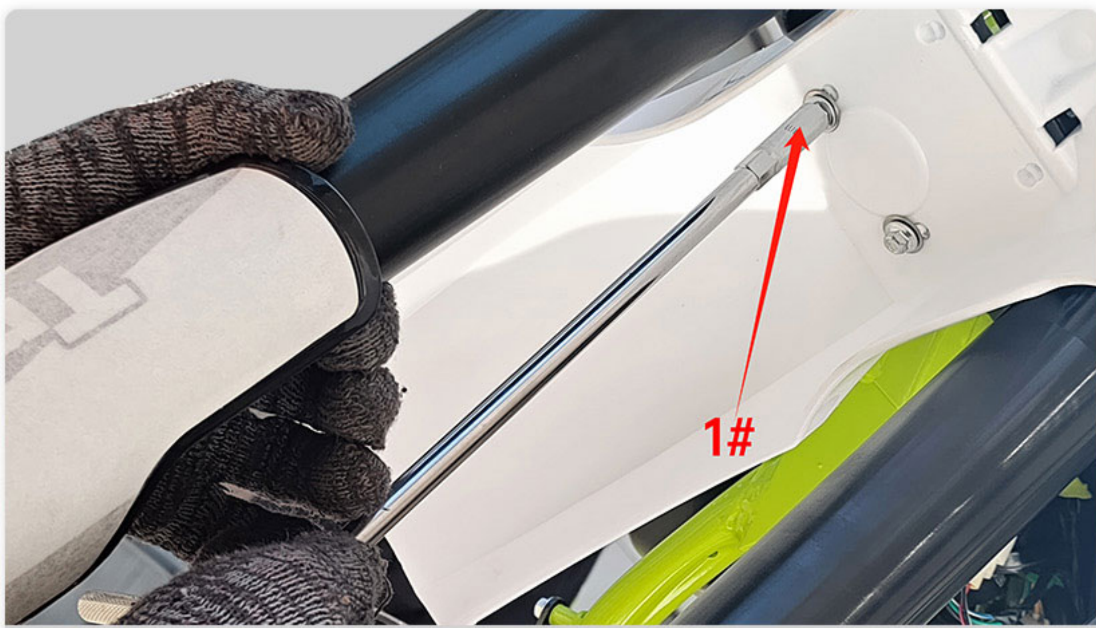
13. Using 1# tool lock 2pcs screws on the bottom of front fender tightly, and lock the screws on graph 12
