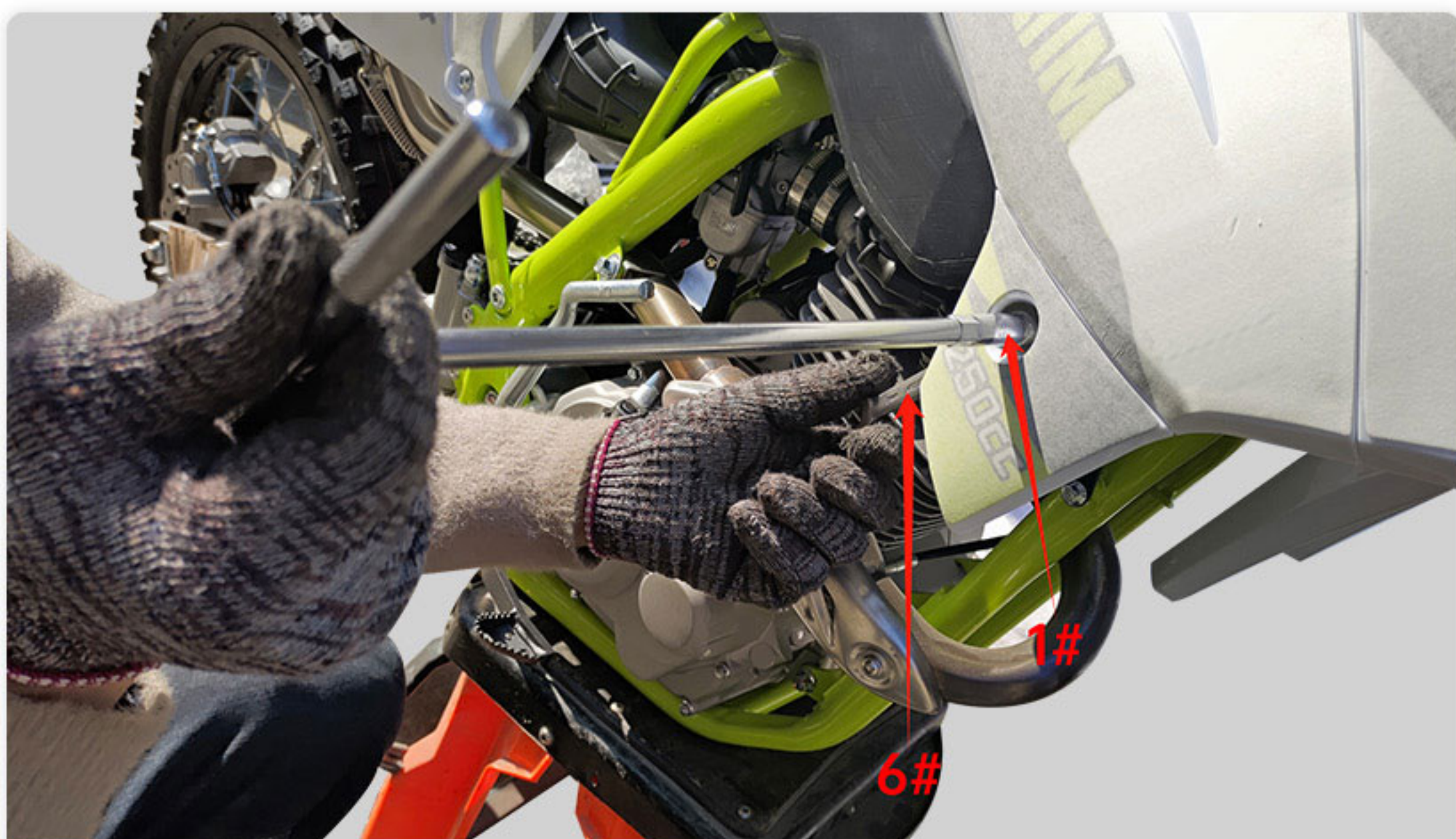
21. Using 1# 6# tool fix the cover with its bracket, lock the screws tightly
