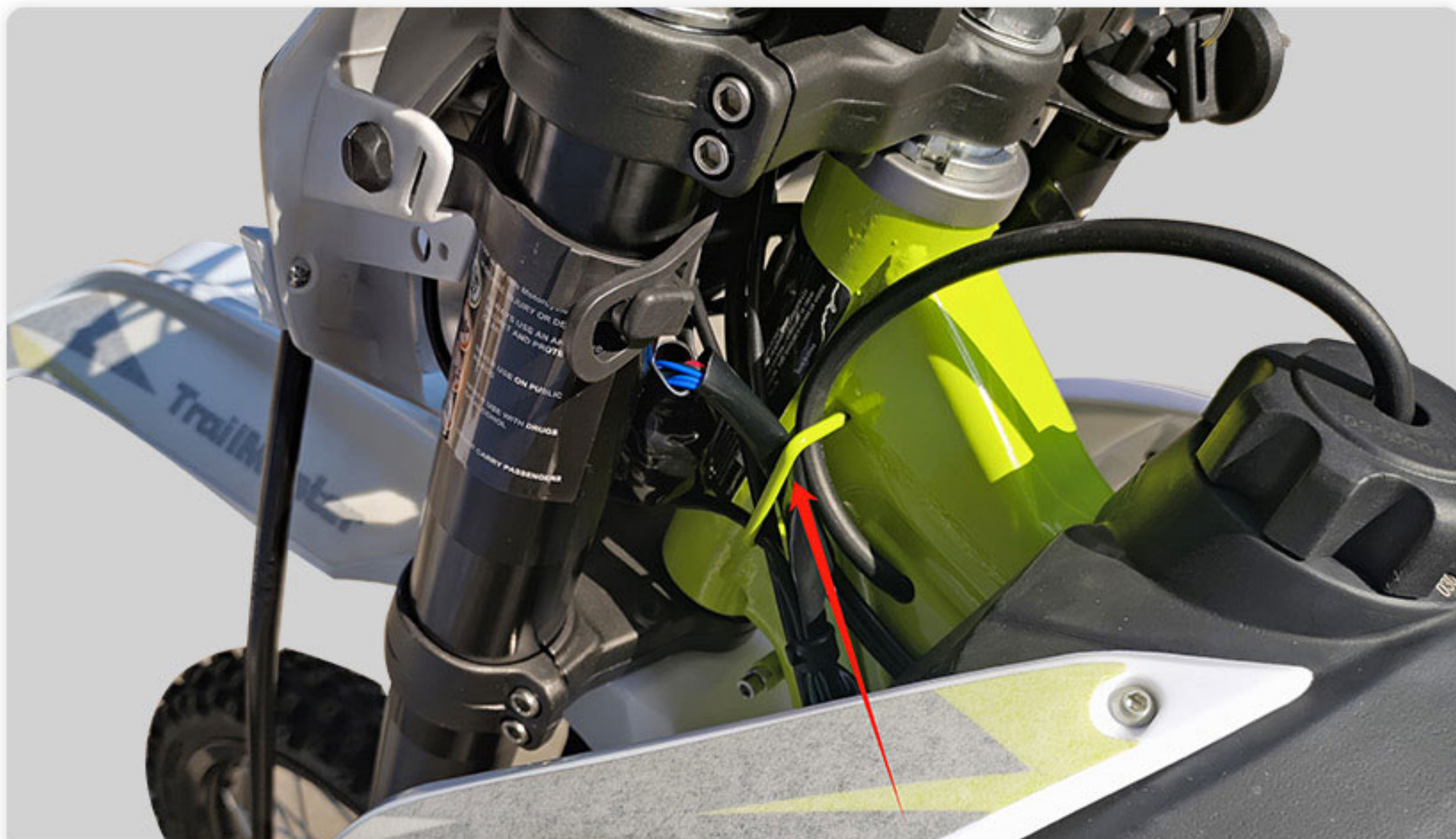
27. Assemble breath hose, protect pad, fix the wires on clip
