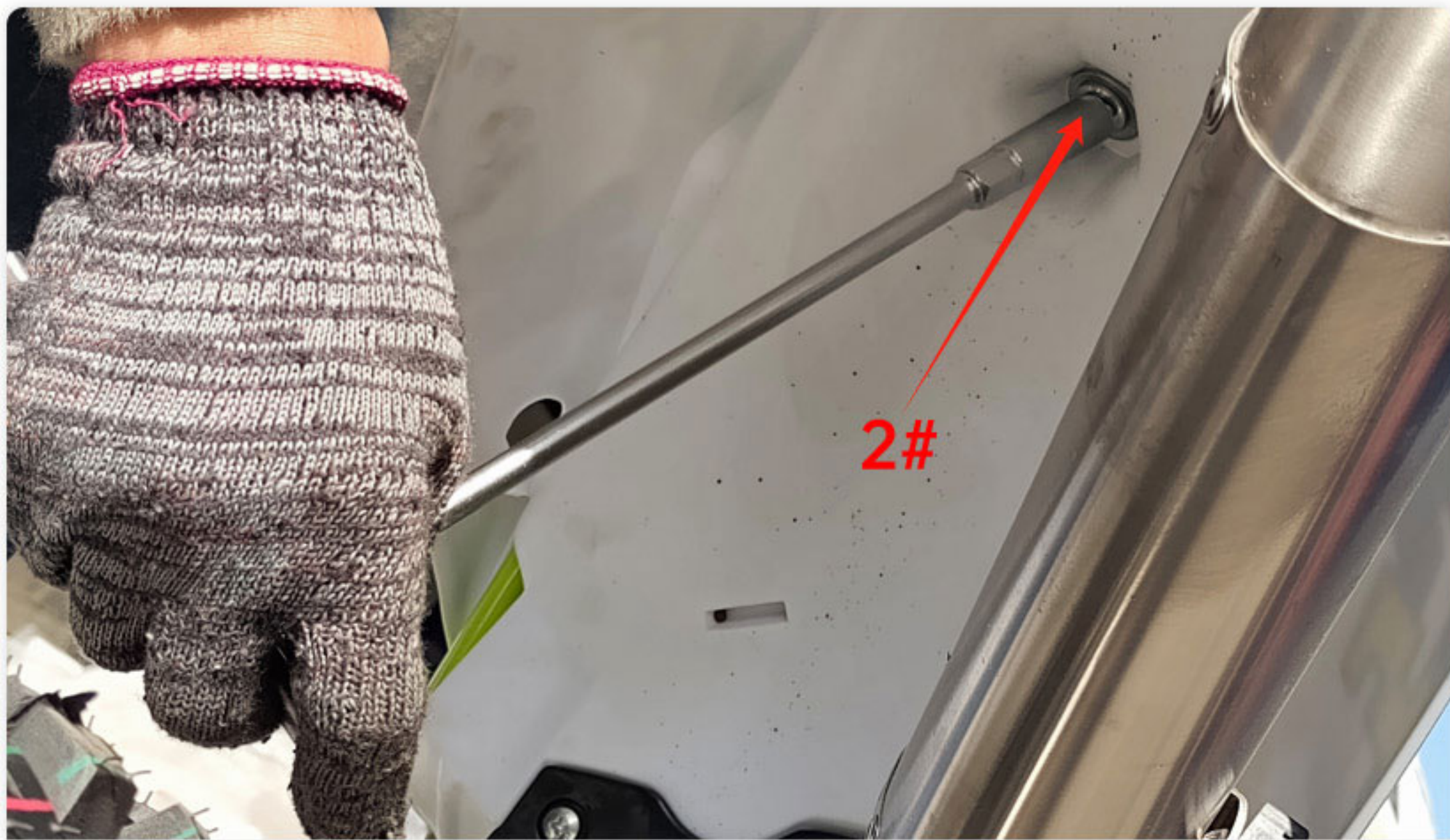
19.Using 2# tool disassemble the screw fixed on seat and open it.
