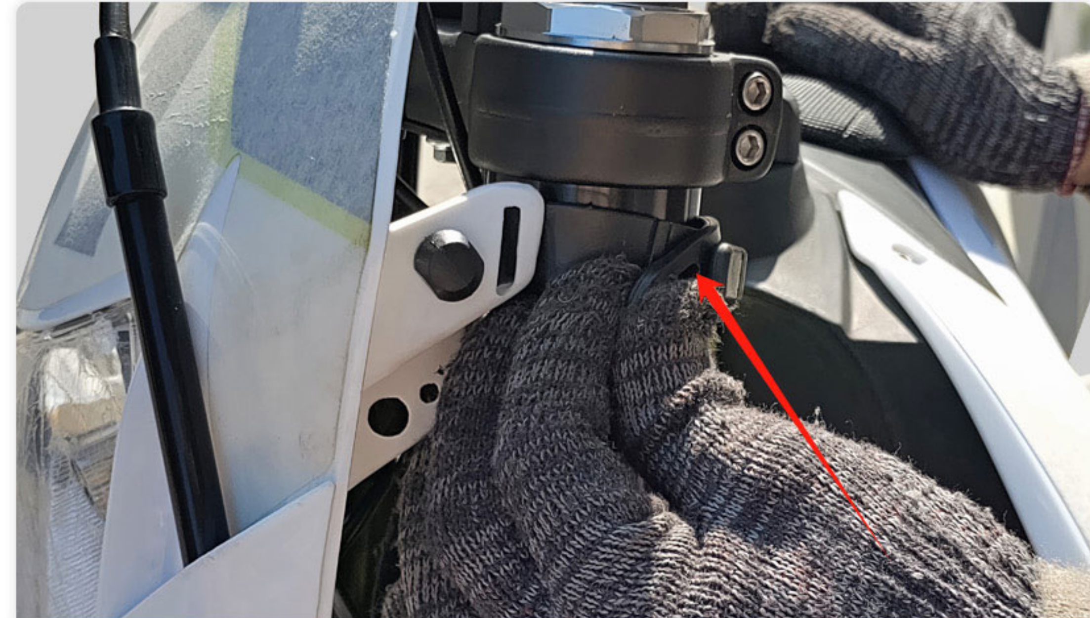
26. buckle the headlight and front fender, fix them on front shock with belt
