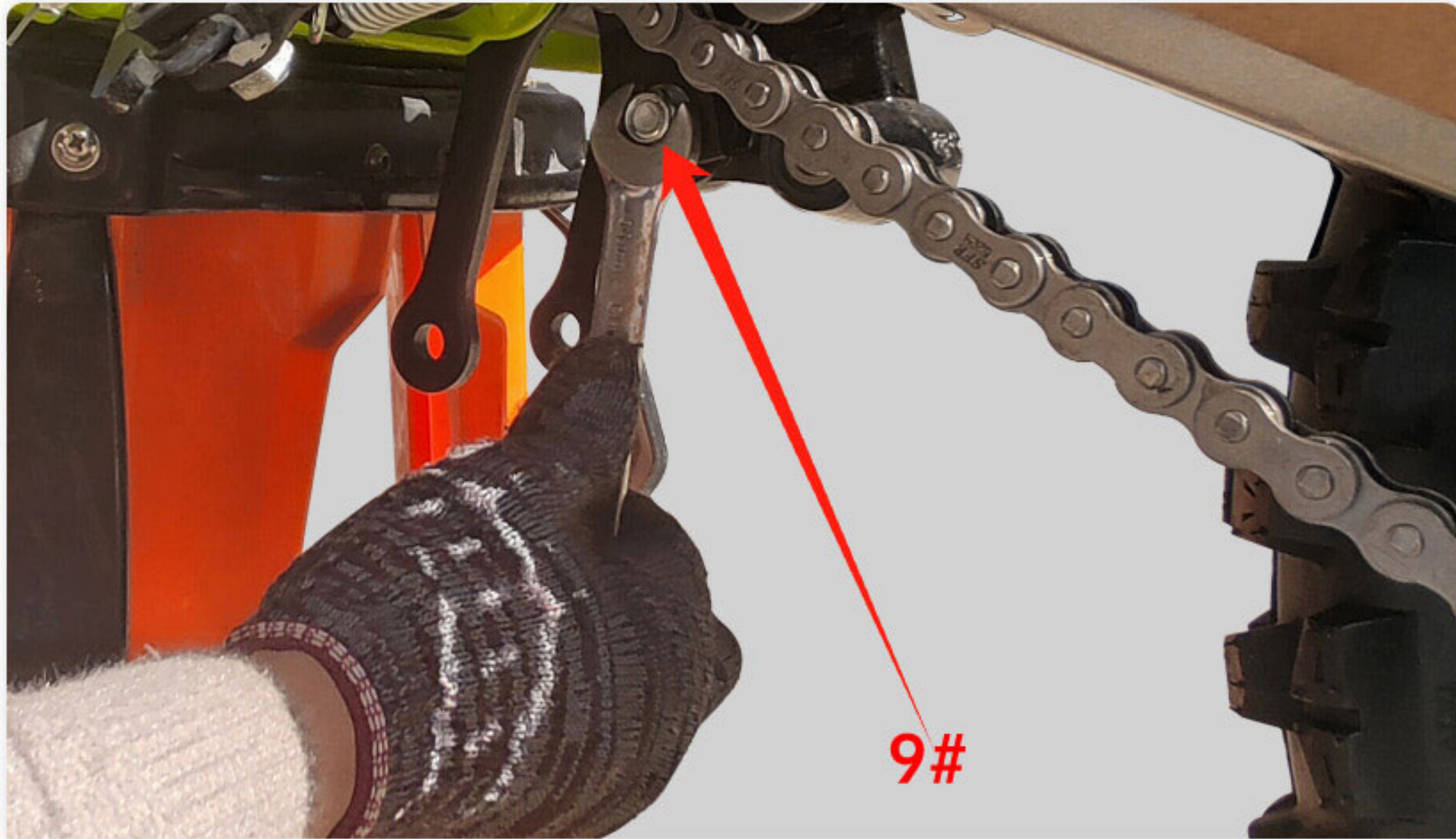
17. Using 9# tool assemble the Rear Suspension and Triangle Lever Linkage,lock the screws tightly
