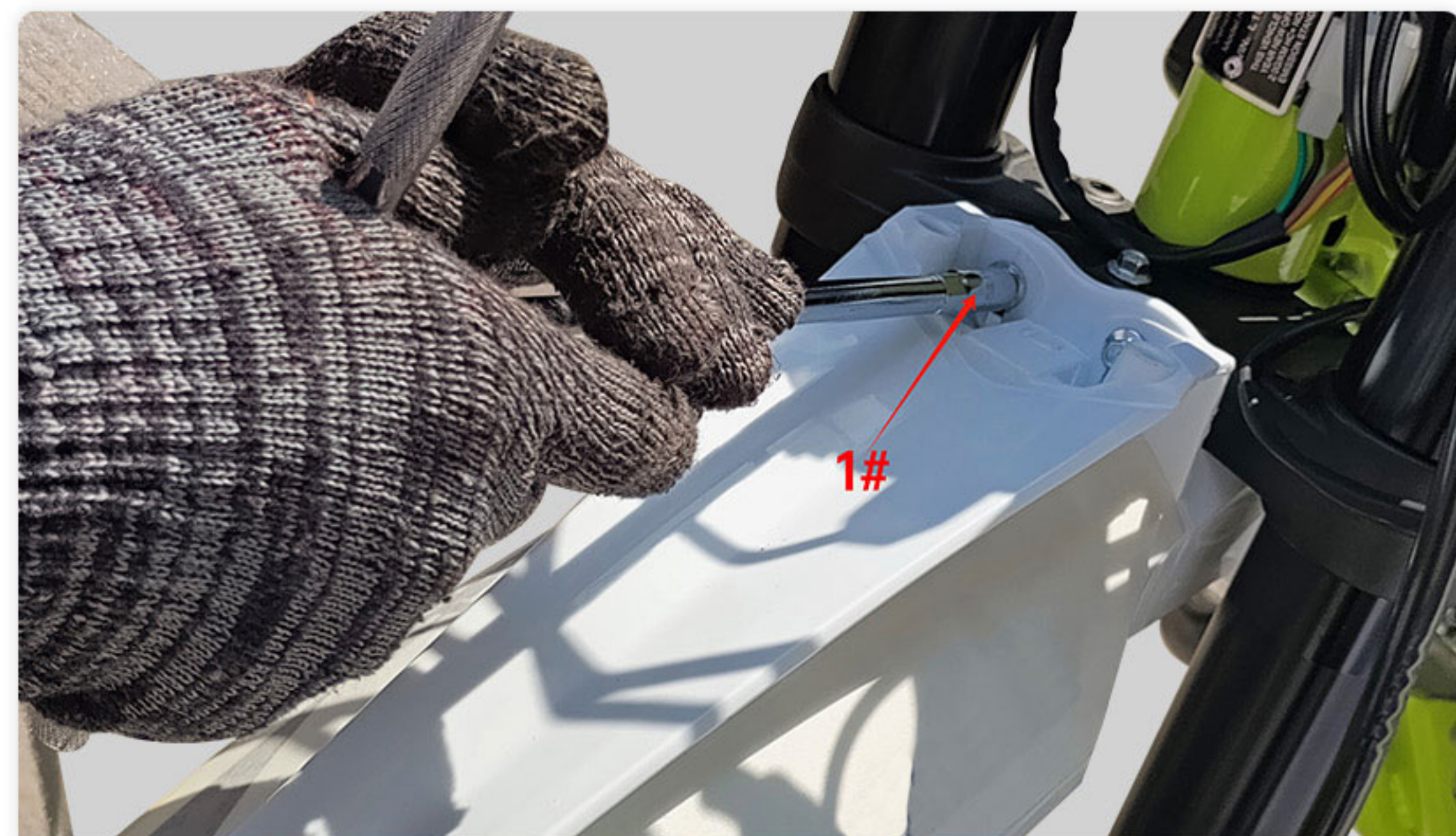
12. Using 1# tool put 2pcs screws on the above of front dender, don't lock tightly
