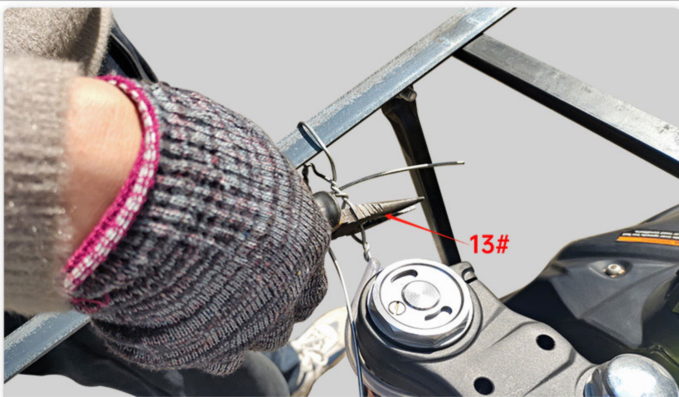
7. Using 13# tool cut the iron wire fixed the dirt bike
