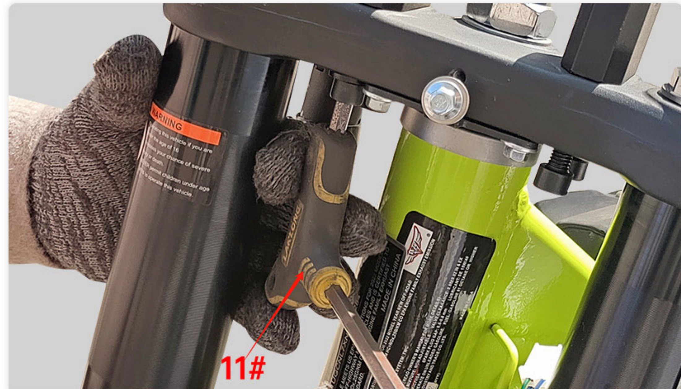
10. Using 11# tool fix and lock the bottom riser and bracket of Ignition Switch with 4pcs screws
