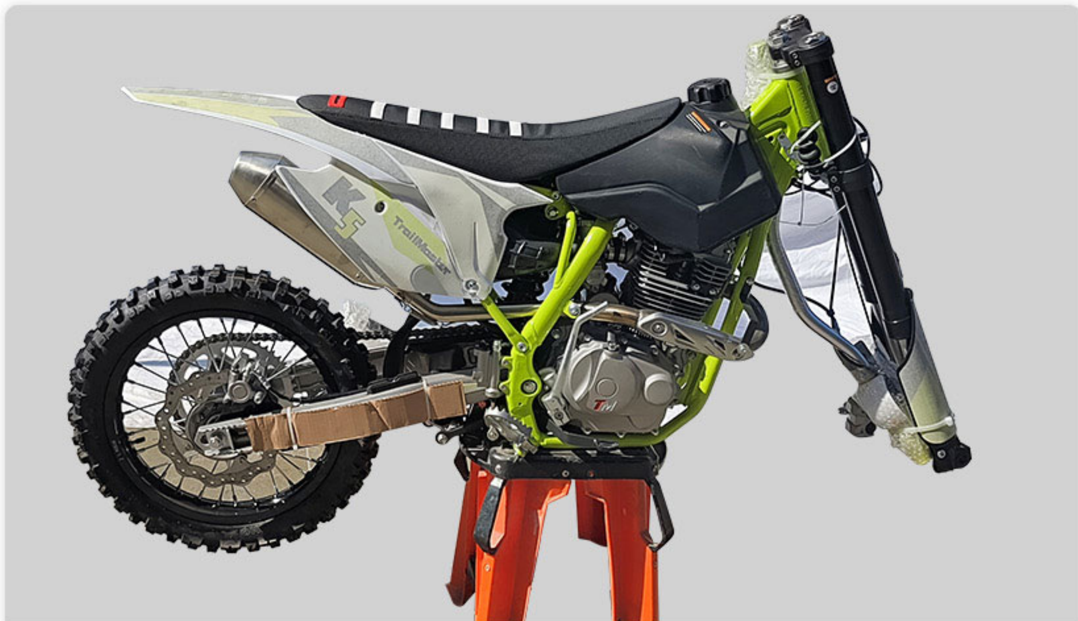
9 .Put the dirt bike body on work chair and fix stably
