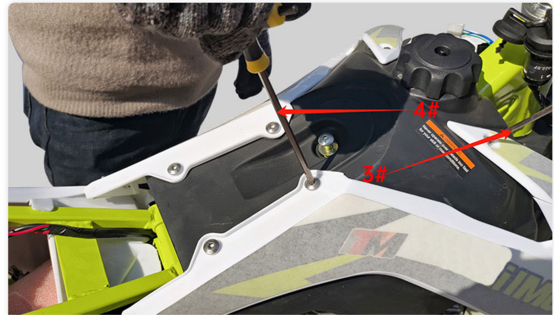
20. Using 3# 4# tool assemble left and tank covers
