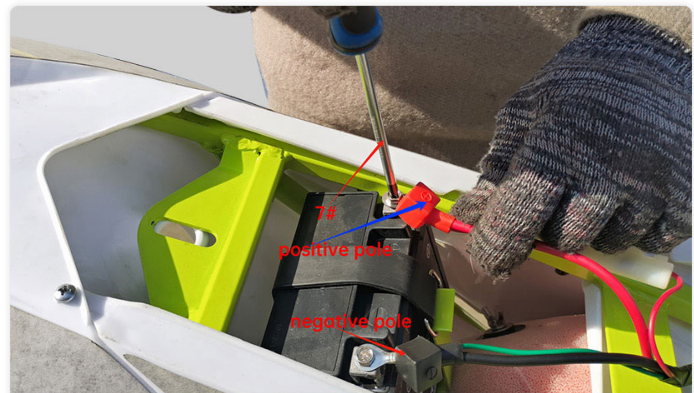
22. Using 7# tool connect the screws on battery as graph
