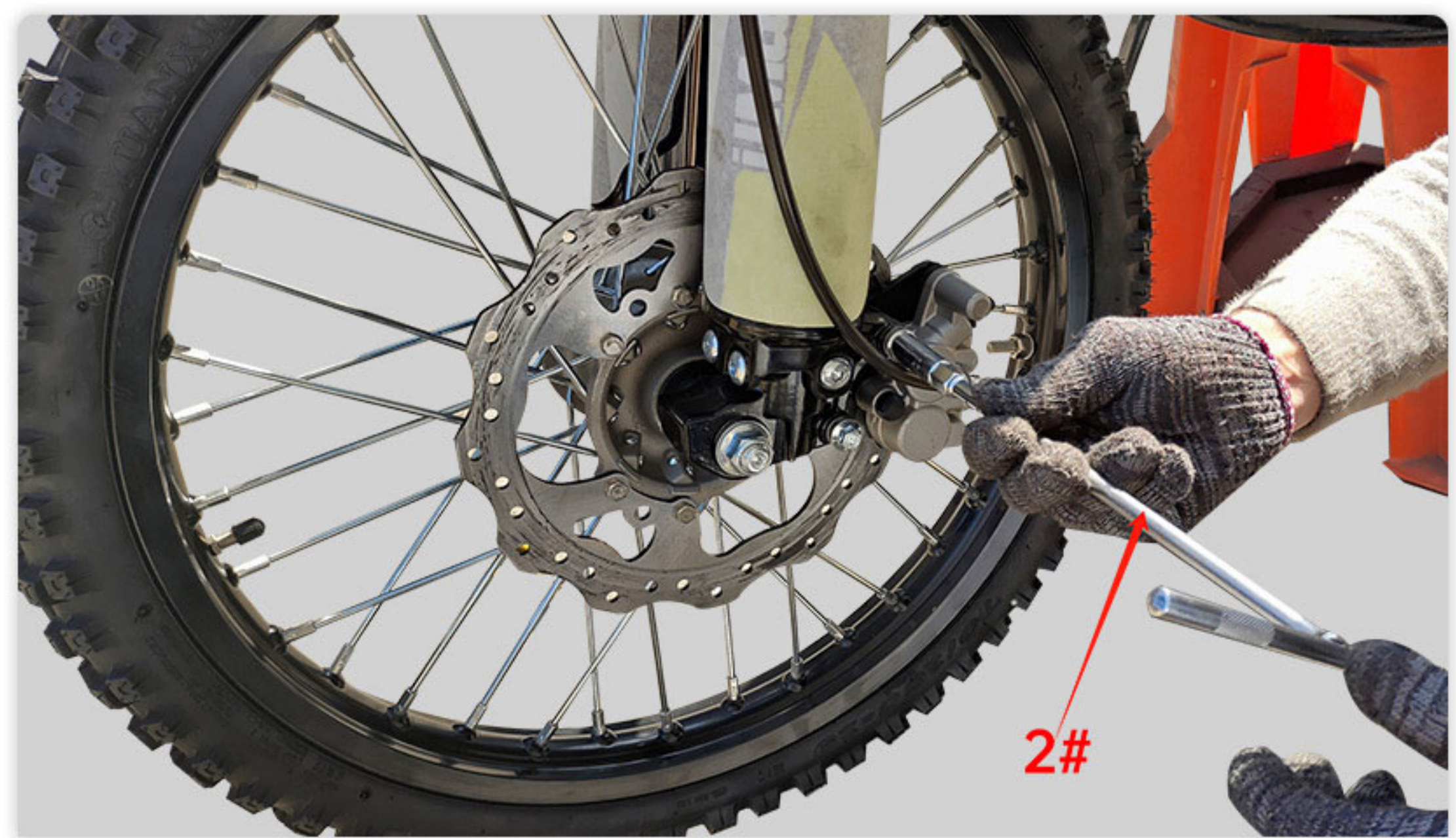
16. Using 2# assemble the front brake caliper, put the brake pad on brake dis, lock tightly with 2pcs screws
