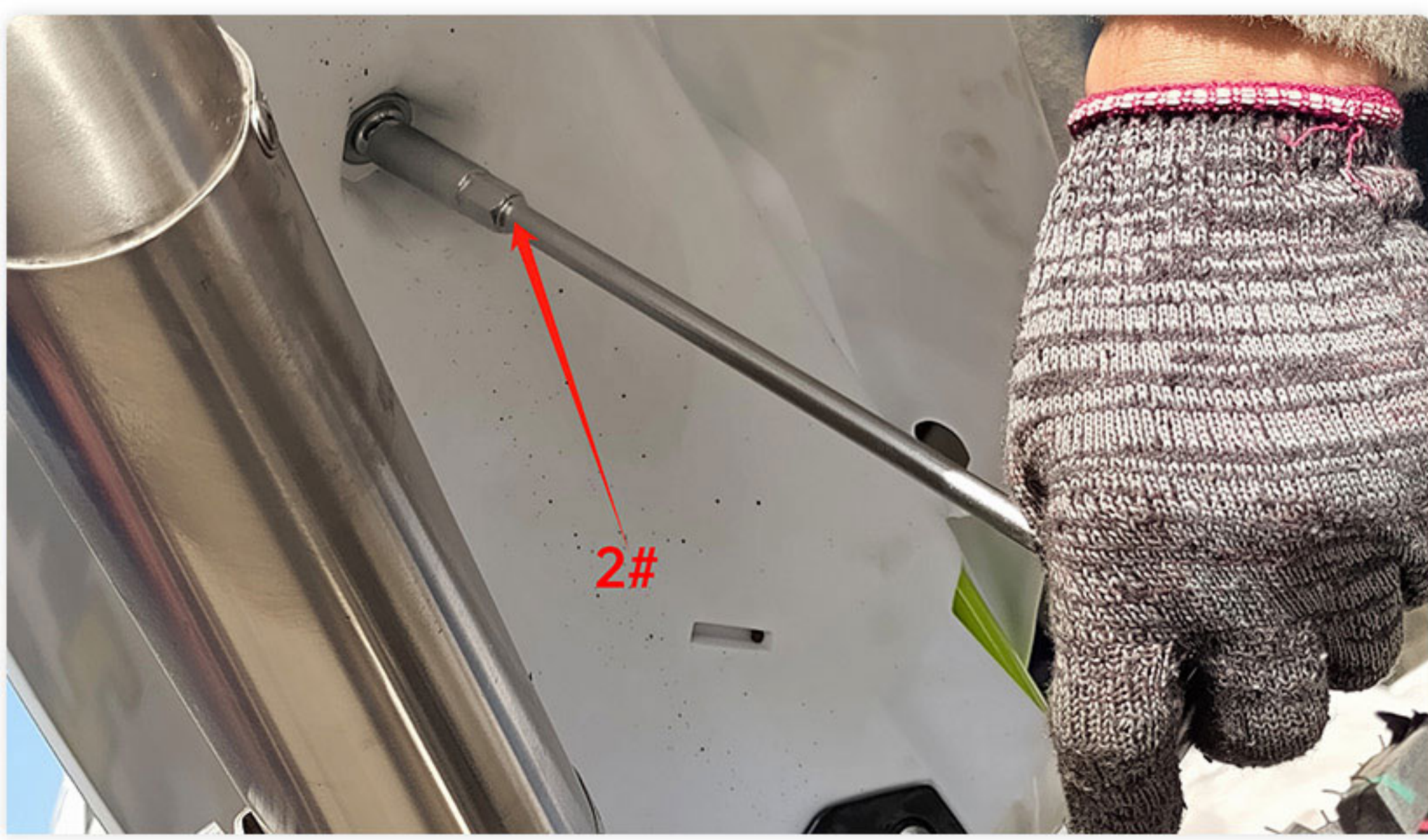
23. Assemble seat, fix and lock the screws of seat using 2# tool
