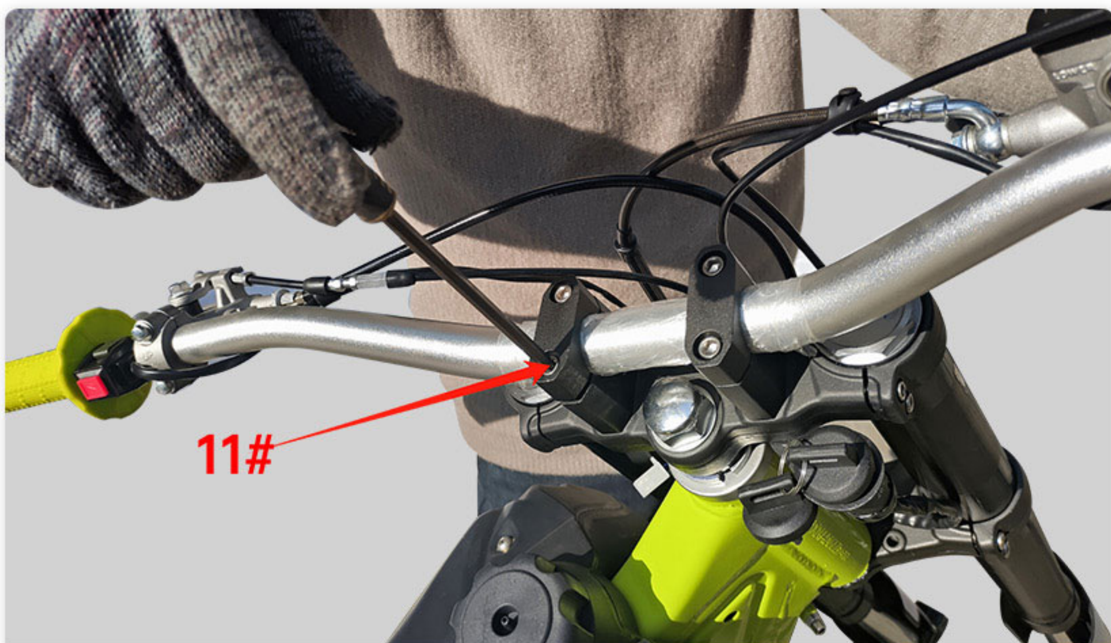
11. Using 11# tool fix the handle bar with 4pcs screws, make spacers of both ends equilly between graph marks
