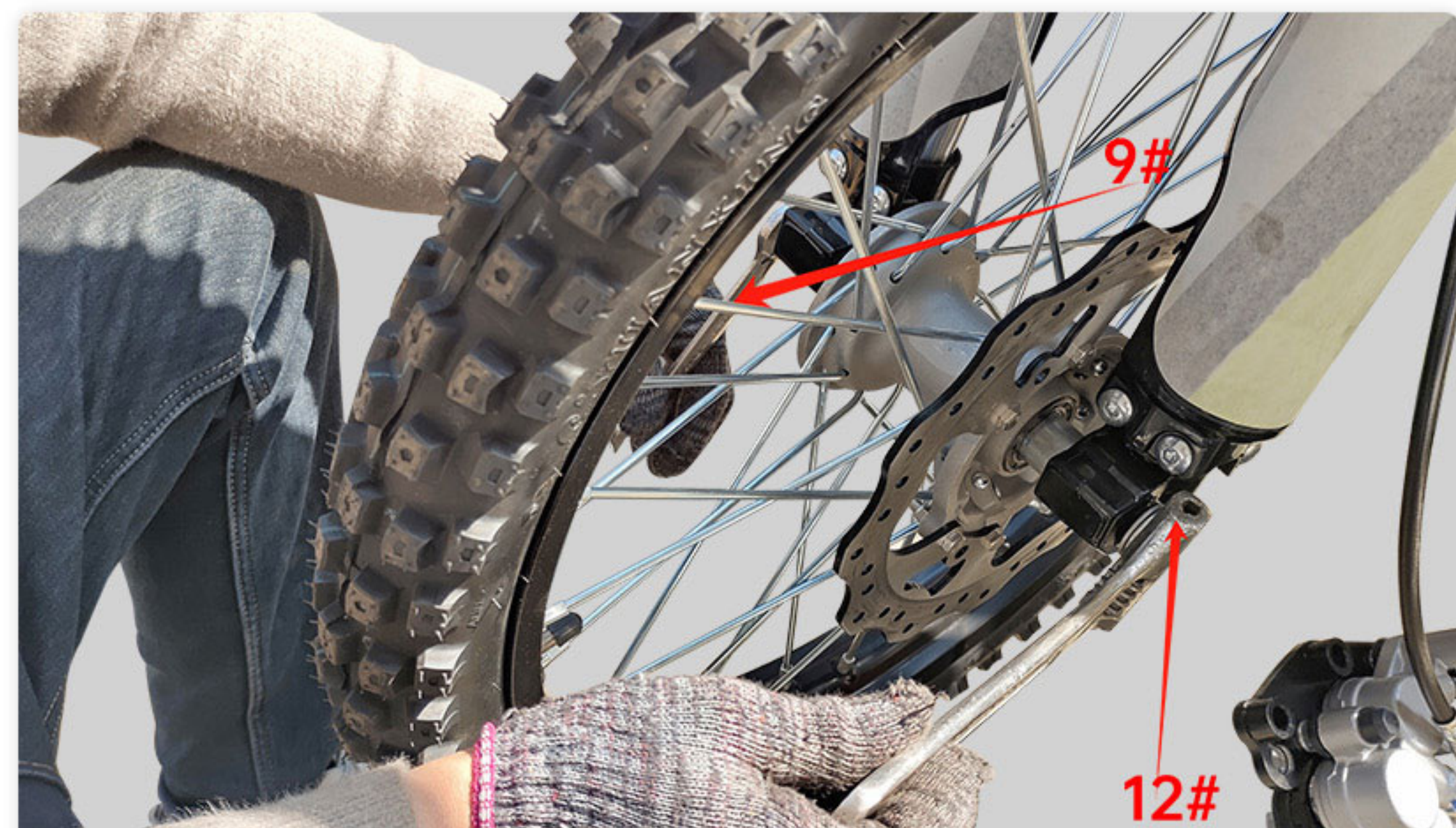
14. Using 9# 12# tools assemble front wheel and lock screws of front axle tightly
