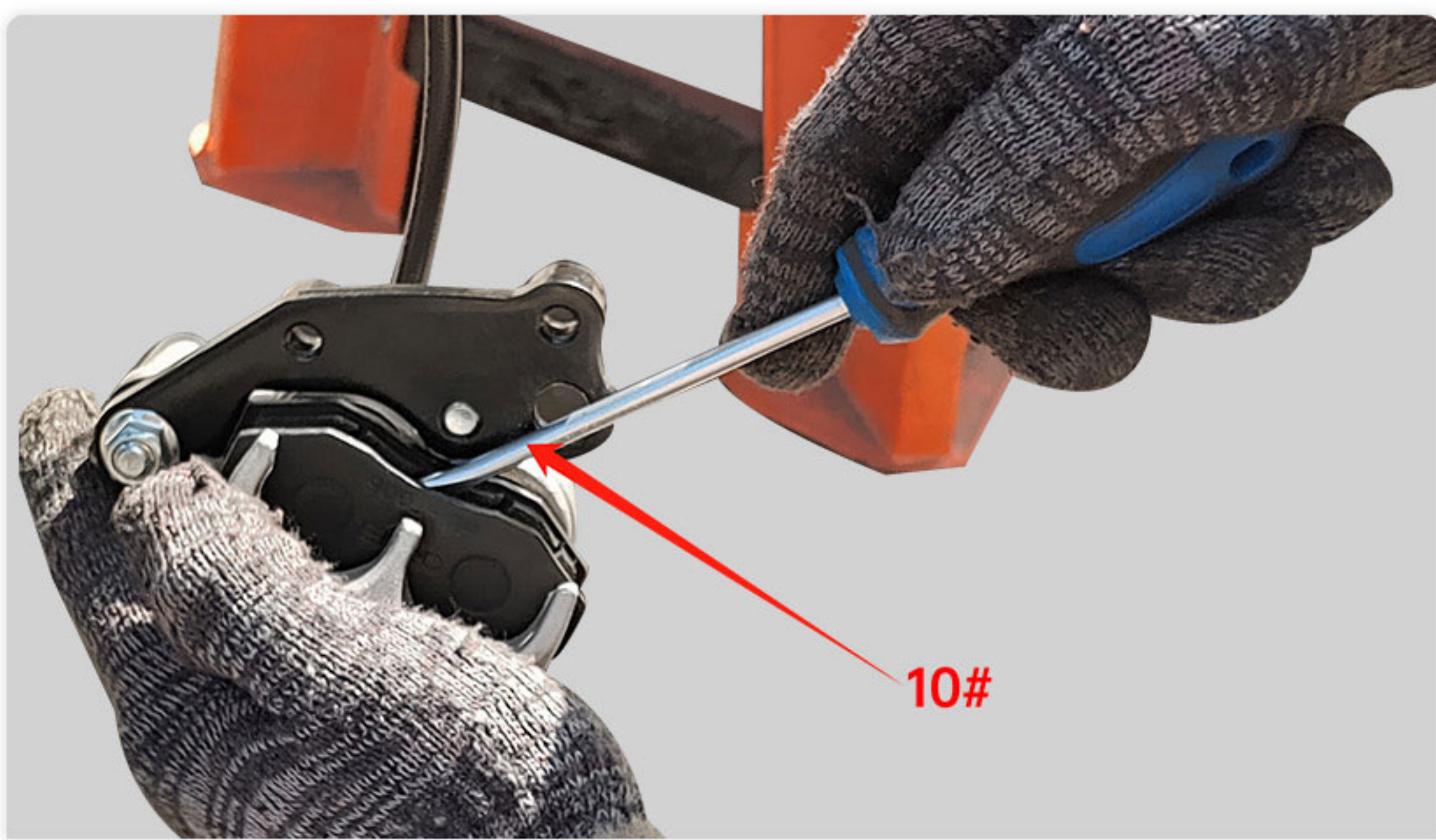
15. Using 10# tool pry the brake pads apart
